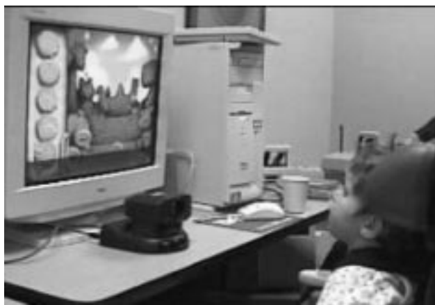
Fig. 3. The Camera Mouse user playing with educational software. The video camera is placed underneath the user computer's monitor.
