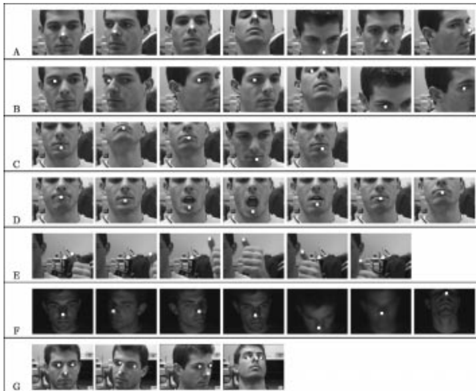
Fig. 7. The eye, nose, mouth, and thumb were tracked to determine features that can be tracked reliably (A–E). Sequence F shows that the nose can be tracked even if the laboratory is dark and only the screen illuminates the user’s face. Sequence G shows tracking of a set of features. Each test sequence contains 1000 images. A representative subset of each sequence is shown. The tracked subimages surrounding the features have been filled white for better viewing. They are 15 pixels wide in sequences A–F and 10 pixels wide in sequence G.
